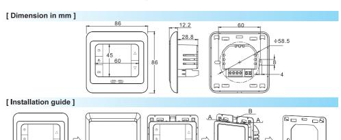
Step 1: Separate the Polycarbonate Bezel unit from the LCD screen.
