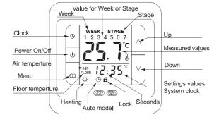
[ Children Lock ] Press key ① \( \mathred{\Pi} \) for 2 seconds at the same time, the controller keypad would be locked. Screen would show \( \overline{\Pi} \). Press the \( \Overline{\Pi} \mathred{\Pi} \) at the same time for 2 seconds under the locked status, keypad would be unlocked.
