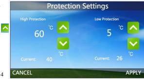
**High Protection:** It uses external sensor to probe floor temp. When floor temp. over set protection temp. the system will be shut off automatically.
